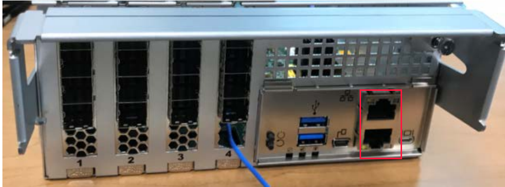
Figure 3.6 RJ45 port on server's operator panel
